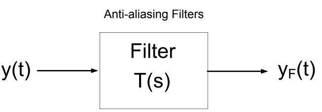
Lowpass filters are widely used to limit the bandwidth of a signal y(t) to the band-edge of the filter before the signal is sampled.
