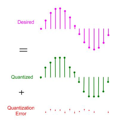
Unwanted signals in the output of a system are called <u>noise</u>.
