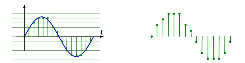
Amplitude quantization introduces errors in the output
