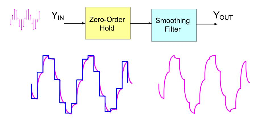
Smoothing filter removes some of the discontinuities in the output of the zero-order hold
