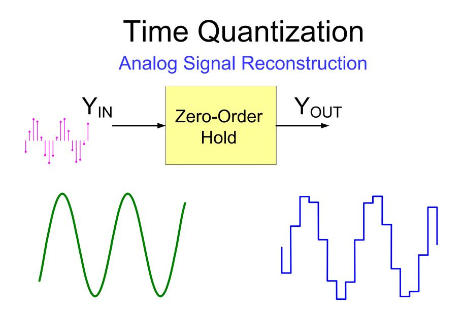
Although Sampling Theorem states there is sufficient information in samples to reconstruct input waveform, does not provide simple way to do the reconstruction
